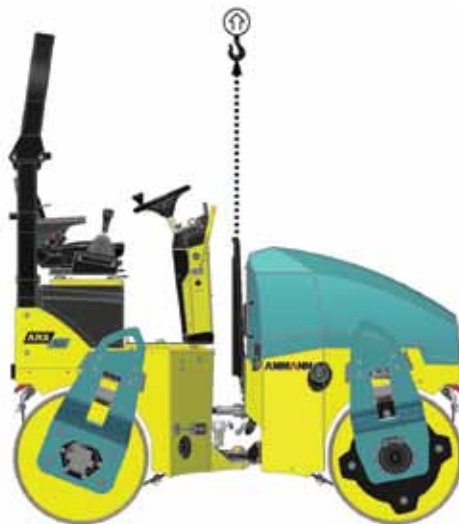
Central lifting point on ARX1(standard) ARX2(option)
