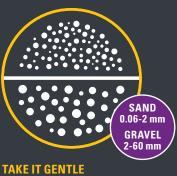
For sand and gravel you can achieve high-density compaction in either a dry or saturated state. The level of compaction depends more on grading than moisture. Too much compaction of sand and gravel is like beating a concrete wall with a sledgehammer. It can crush the material and reduce the load bearing capacity.
